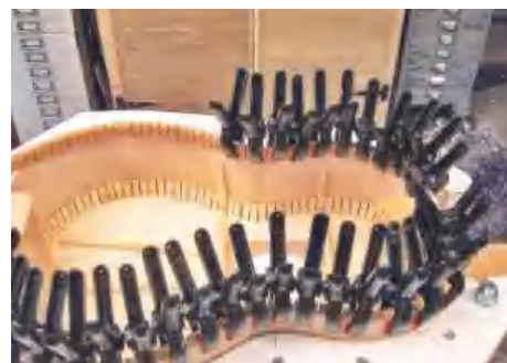
STEP 32. Clamping the kerfed lining into place
